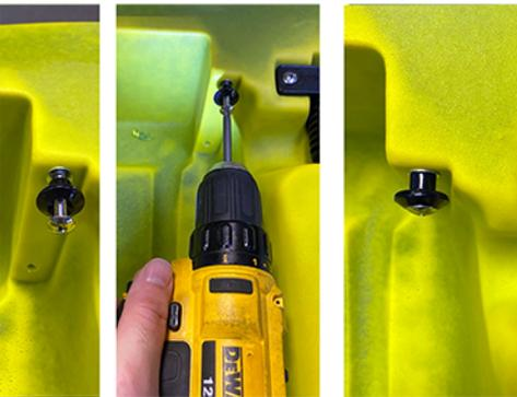
**5.** Place the phillips head bolt and deck fitting assembly into the flanged tapping insert on the Staxx. Tighten with phillips head bit (or screwdriver), taking care not to overtighten. The bolt and deck fitting will not be flush to the side when installed (see photo).
