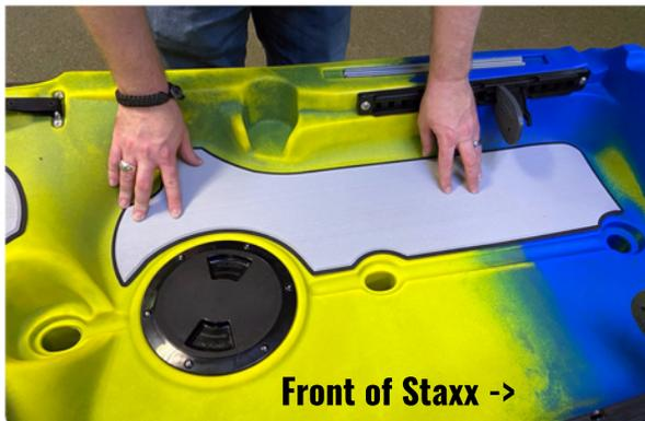
2. Clean and wipe down deck pad area with rubbing alcohol prior to application.
