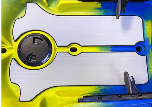
4. Heat deck area with either a torch or a hair dryer. Remove backing from deck pad and apply heat to adhesive. Slowly press down pad, starting at the end and working toward the opposite end. If bubbles occur, simply slice with a razor blade to release air.
