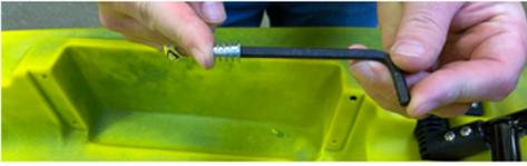
**3.** Place a flanged tapping insert (I.) on the end of the provided 5mm hex key. Align insert with the drilled hole and tighten with key until flush with the side of your Staxx.
