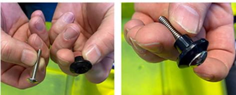
**4.** Next, place a 10-24 phillips head bolt (L) through an open deck fitting (J).
