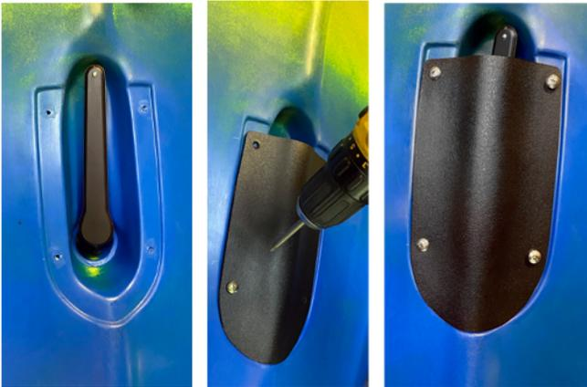
**4.** If installing a transducer, feed transducer wire through scupper hole so transducer sits flush in the transducer scupper pocket. Place transducer cover over transducer and use the four Phillips head bolts that were removed earlier to bolt the transducer cover onto your Staxx, lining your bolts up with holes in both the cover and the kayak.
